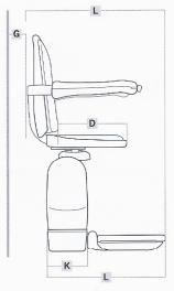
Power Supply Maximum Capacity Track Mains Supply 24V DC (battery) 280lbs (optional 350lbs) Extruded Aluminium 120V AC, 1.5 Amp Charger
